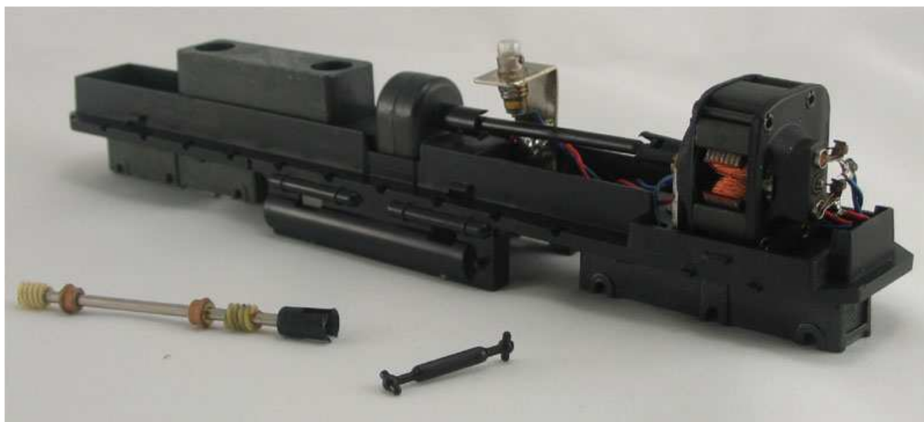
Phase I chassis, with truck drive shafts removed
