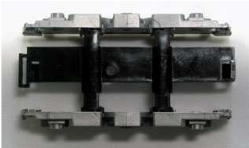
Early PowerTorque truck sideframe cap, with slot for removable coupler pocket
