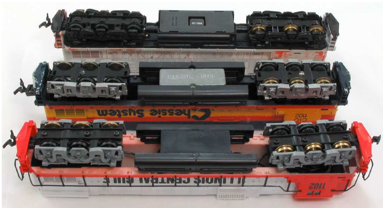
Fuel tanks, top to bottom: Phase I, Phases II and III, and Phase IV
