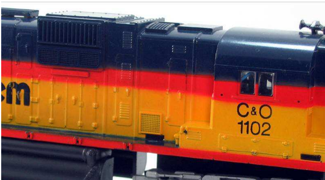
Note how the first double-door's hinge does not go to the bottom...
