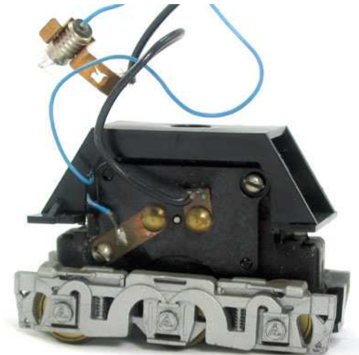
“Mark I” Powertorque motor truck, with closed cover
