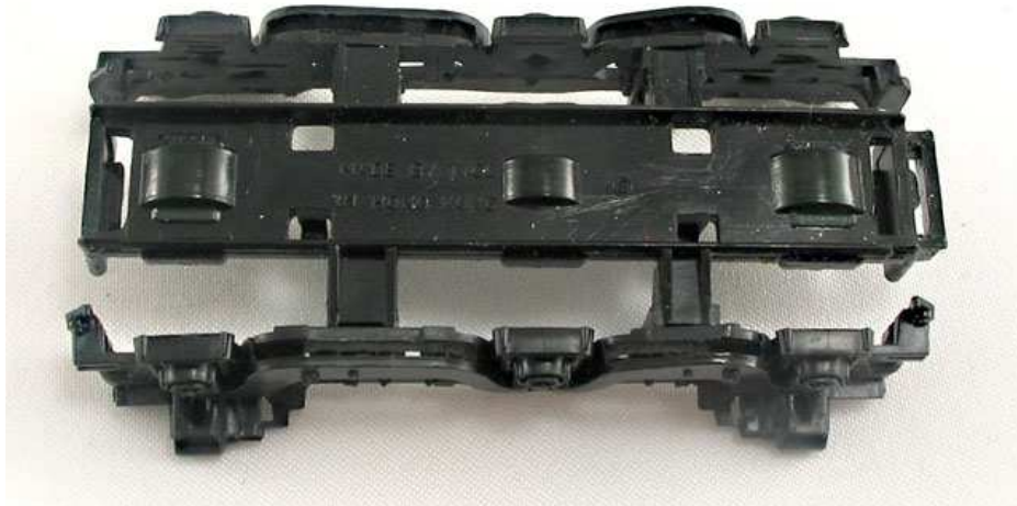
Phase I Truck Sideframe drive cap. Note the pocket on the right end.
