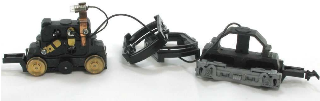
Revised, Powertorque "Mark3" drive.
