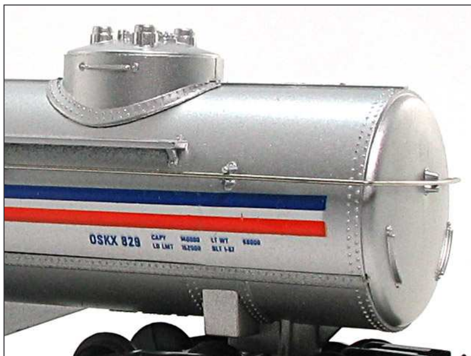
The build date says "1967", but tank cars hadn't been riveted for over a decade!
