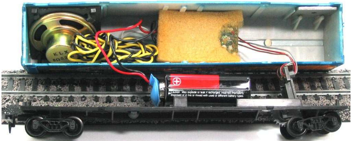
Sound of Steam components layout
