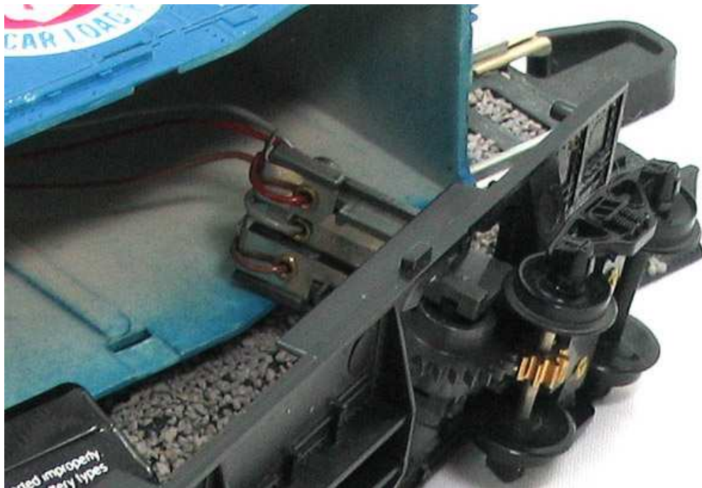
Closeup of module truck unique to #957 Electronic Sound car
