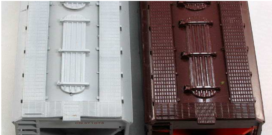
Hatch details. Note the more-defined hinges and strap rivets on Tyco's (right) Even the roof walks are slightly different.
