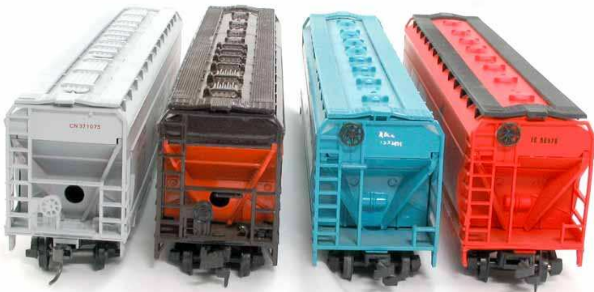
Comparison of end details. Athearn & Tyco have the same ladder rung and brake gear arrangements; AHM/Bachmann differ greatly and also omit the access hole in the end panel.
