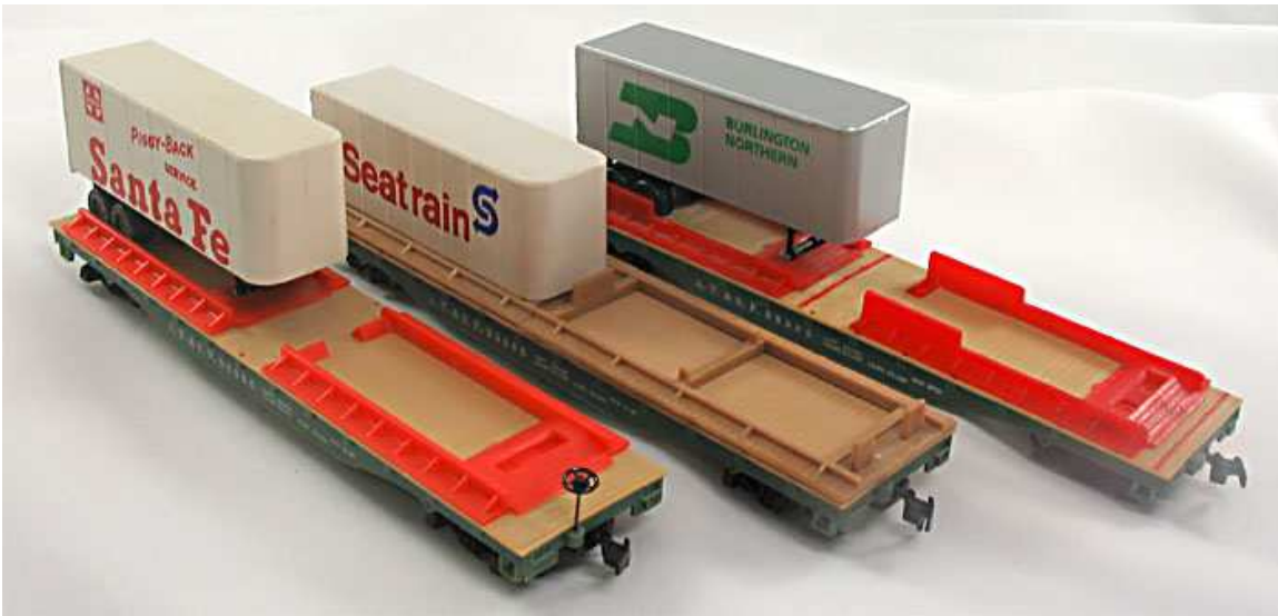
Left to right: Piggyback cradle; Container cradle; Unloader cradle 2 on line-painted deck.
